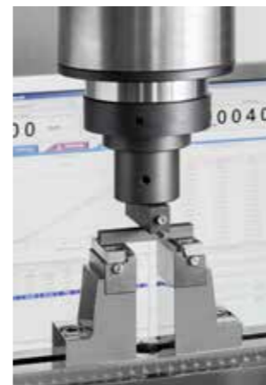
Flexural test (Universal testing machine)
