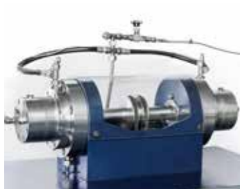
Mechanical seal test rig
