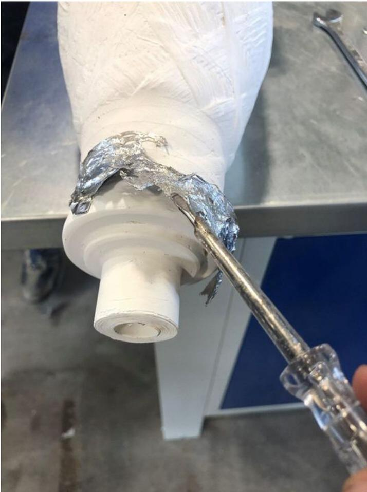
Figure 2: Solidified Aluminum melt from OFC materials can be easily removed from a dosing container.
