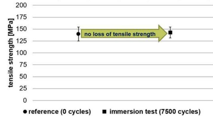
Figure 3: There is tensile strength for OFC specimens after immersion tests in AlSi9Cu3 alloy.
