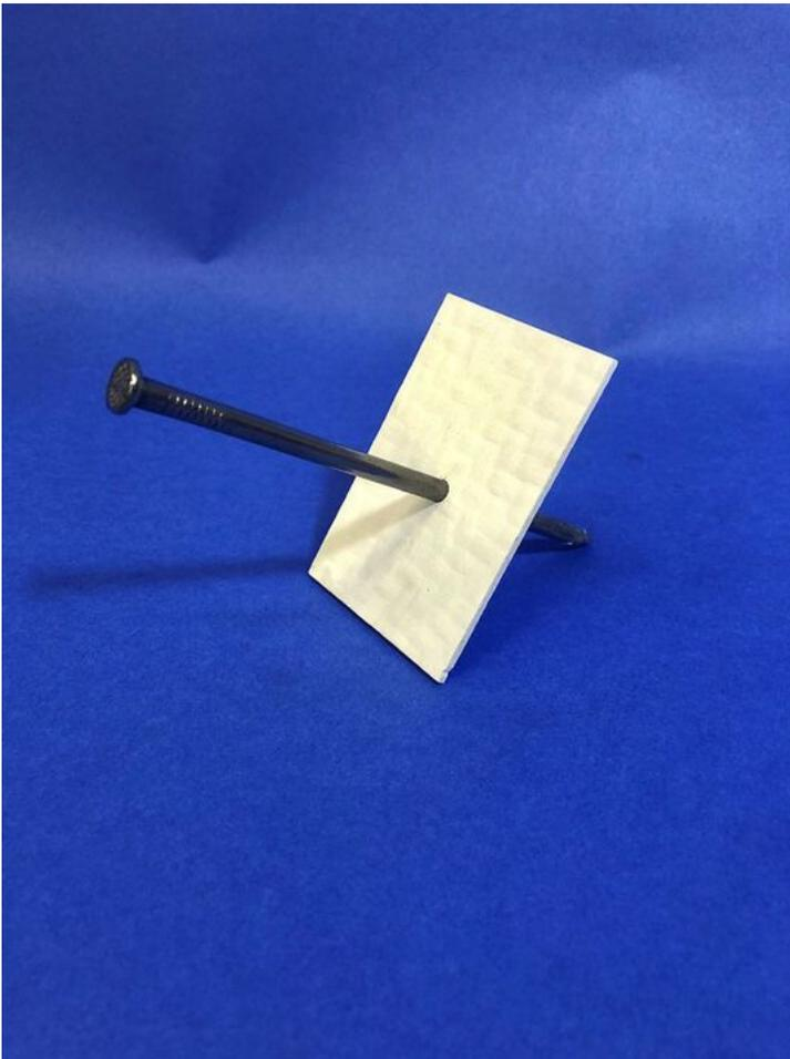
*Figure 1: Local breaches on the component do not lead to overall system damage as can be demonstrated by the crack-free puncturing of a nail through an OFC panel.*
