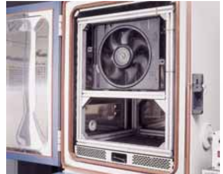
Climatic chamber made by Weiss-Klimatechnik (Schunk Group). Regulation of humidity between 10% - 95% is possible, the temperature can be adjusted from -40 °C to +180 °C
