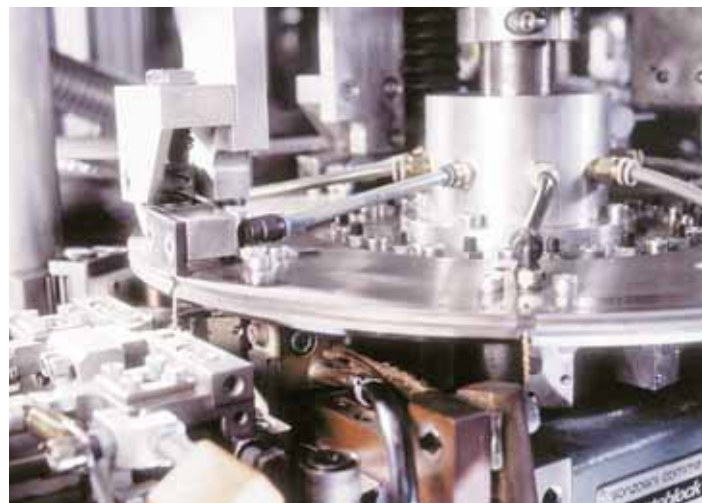
automatic linear grinder LIN NT 2 and rotary table, fully automatic machining of carbon brushes
